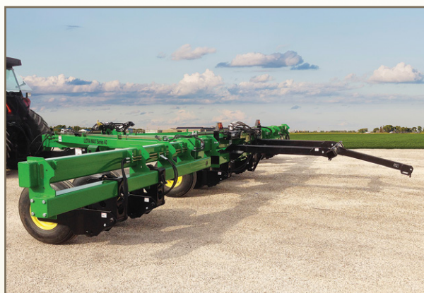
Optional rear Heavy Duty Drawbar Hitch - self leveling
