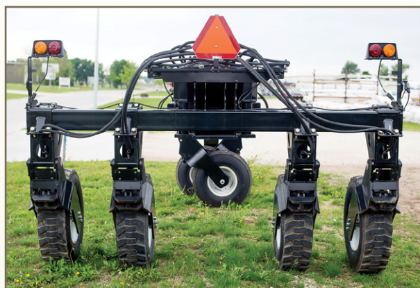
Standard Tire Set-up (folded) and Road Safety & LED Lights (Center tires: Bartread 305/70R 19.5 / Wing tires: Bartread 12.5X/16.5)
