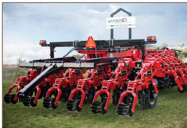
Optional 6 ton on-board storage deck & HD drawbar hitch. (shown on an Ultra Max™ ST4030-8)
