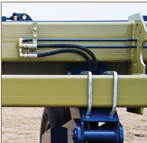
Adjustable wheel units & easy access hydraulic lines
