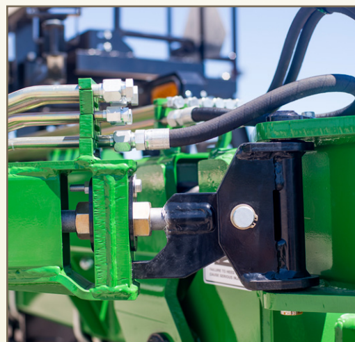
Draft tube adjustment w/ nut keeper (located next to the wing to eliminate potential tire-turning damage)
